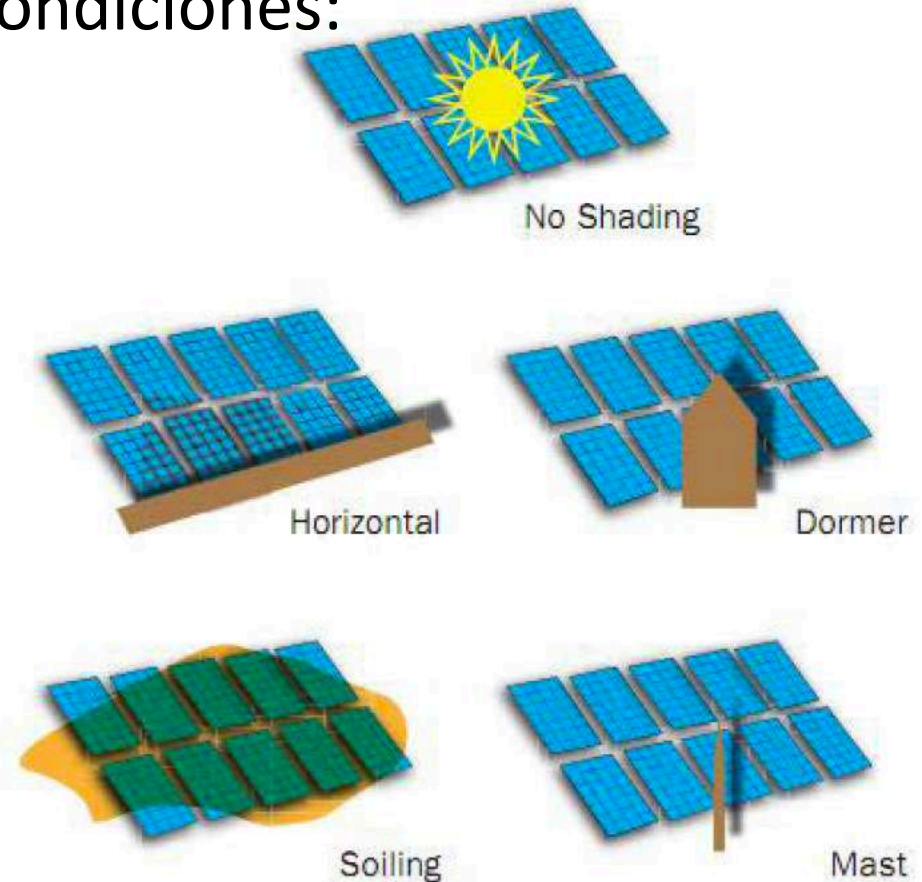
Figure 1. Example obstruction shading conditions Source: PHOTON, November 2010.
